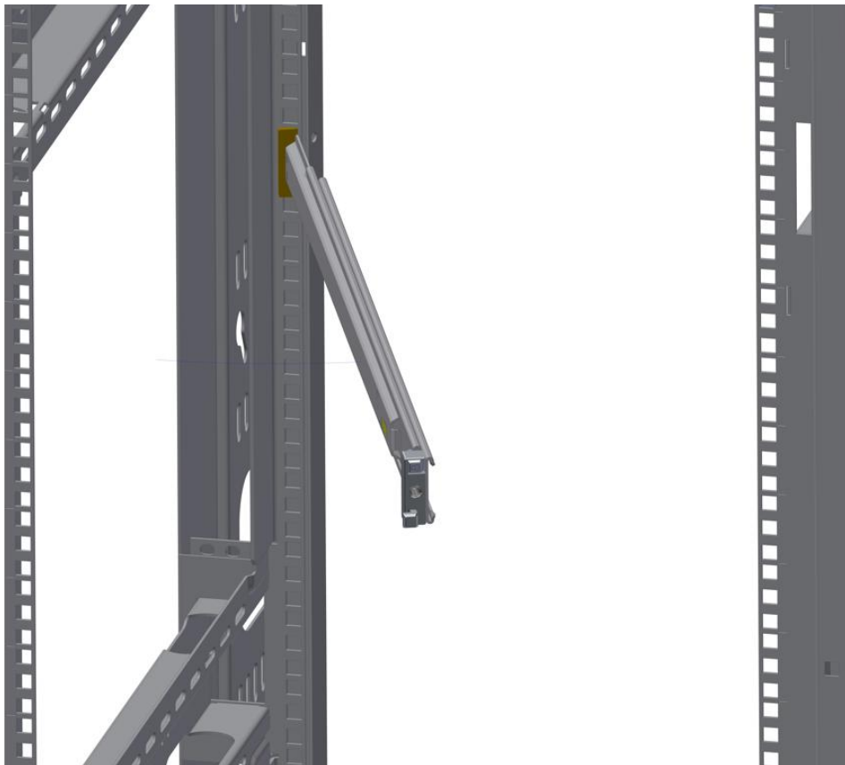
Inserting the Rack Rails (B)
