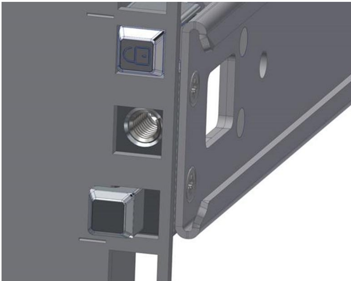
Rack Rails Fully Inserted and Locked in the Rack Assembly
