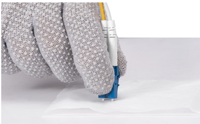
Figure 20: Cleaning Optical Fibers with Special Cleaning Tissues
