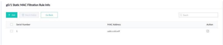
Figure 6: Setting static MAC filtration entries
