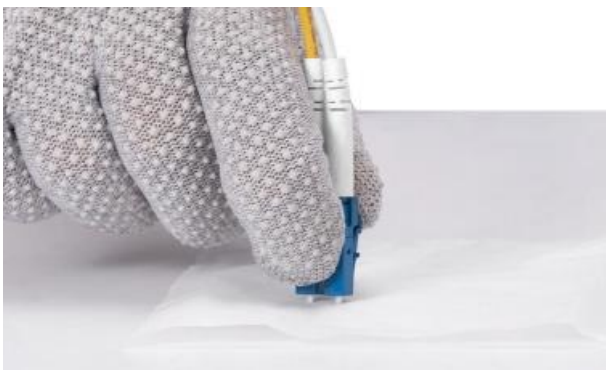
Figure 19: Cleaning optical fibers with special cleaning tissues
