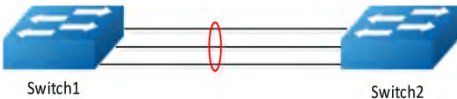
Figure 3-23 Master-slave mode link aggregation
