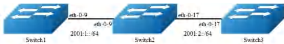
Figure 14-1 ipv6 unicast routing
