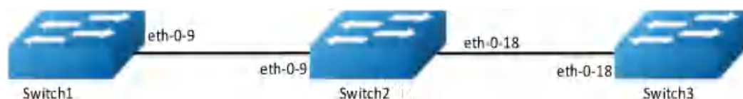
Figure 10-3 PTP Timing Domain
