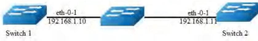
Figure 17-52 Static Route Track
