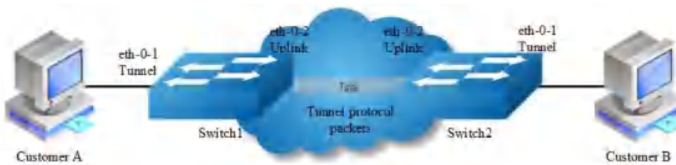
Figure 3-33 L2 protocol tunnel
