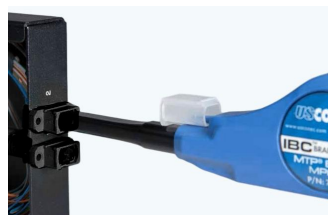
Push cleaner into adapter until click confirms completion
